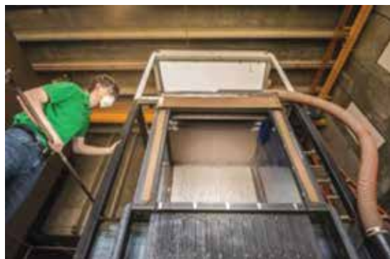
Joshua Mark Christian working with the falling particle receiver, which more efficiently converts the Sun's energy into electricity in large-scale, concentrating solar power plants. (Credit: Randy Montoya)
