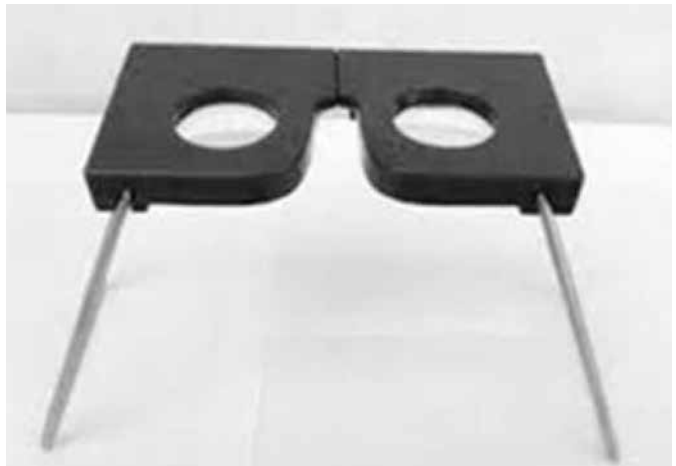
Figure 3. A simple lens stereoscope
